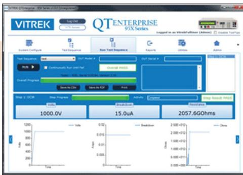
Vitrek's combination cable/harness test solution includes a 950X Series hipot tester, a 964i switch (below) and QT Enterprise software (screen capture).
