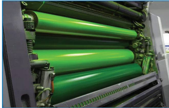
Figure 1. Calender Rollers where consistent gap across the rollers are vital to finished product quality
